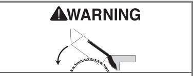
Keep the blade guard installed and in the down position. Failure to do this could result in serious personal injury or death.
